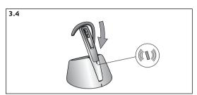
3.4 Place the headset in the charge cradle and charge for a minimum of 30 min. before use. A full charge takes about 2 hours. The visual indicator on the headset will flash green while headset is charging, and the light will remain steady green when fully charged. The same procedure is to be followed when using the travel charger.
