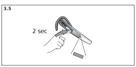
**3.5** Turn the headset on by pressing the Answer/End button for 1 sec. (the visual indicator will flash blue four times and headset will beep three times), or by placing headset in charge cradle. Turn the headset off by pressing the Answer/End button for 2 sec. (visual indicator will flash blue four times and headset will beep three times).
