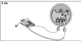
**3.2a** Connect the enclosed telephone cord to the now empty handset port on the telephone, and to the port on the base unit marked with **3**.
