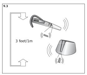
**9.3** Make sure headset and the base are within 3 feet/1m of eachother. When pairing is successful,both visual indicators will flashblue 5 times, and the visual indicator on the base unit will turn to steady green.
