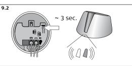
**9.2** Then press the reset button on the base unit for 3 seconds. The visual indicator on the base unit will turn steady to blue.
