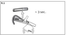
**9.1** At start-up, press the Answer/ End button down for three seconds. Alternatively, remove the snap-on cover and press the reset button on the headset for three seconds. The visual indicator on the headset will turn to steady blue. <sup>1)</sup>
