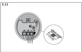
**3.11** Adjust the outgoing volume using the transmit volume control on the base unit. Move the switch through the 3 settings until test person confirms the appropriate volume. <sup>1)</sup>
