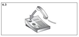
**6.3** To end the call, tap the Answer/ End button on the headset and replace the handset in the cradle, or press the telephone's "end call" button if the base is connected directly to the telephone's headset port.
